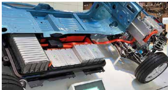
A Nissan Leaf 30 kWh battery pack has 92 cells and weighs 640 lbs.
