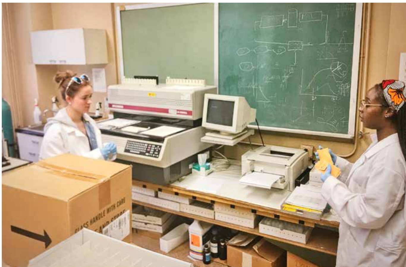
RSO lead technical assistant Emaya Moss (right) worked with RSO technical assistant Margaret Blouin on preparation of swipe samples and operation of a liquid scintillation counter.
