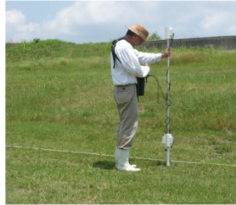
Figure 2. LGS proton precession magnetometer in gradiometer configuration.
