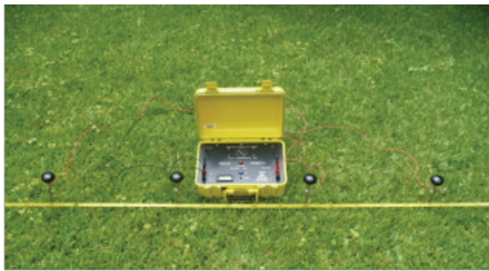
Figure 1. LGS resistivity and IP meter with electrodes arranged in a Wenner array.
