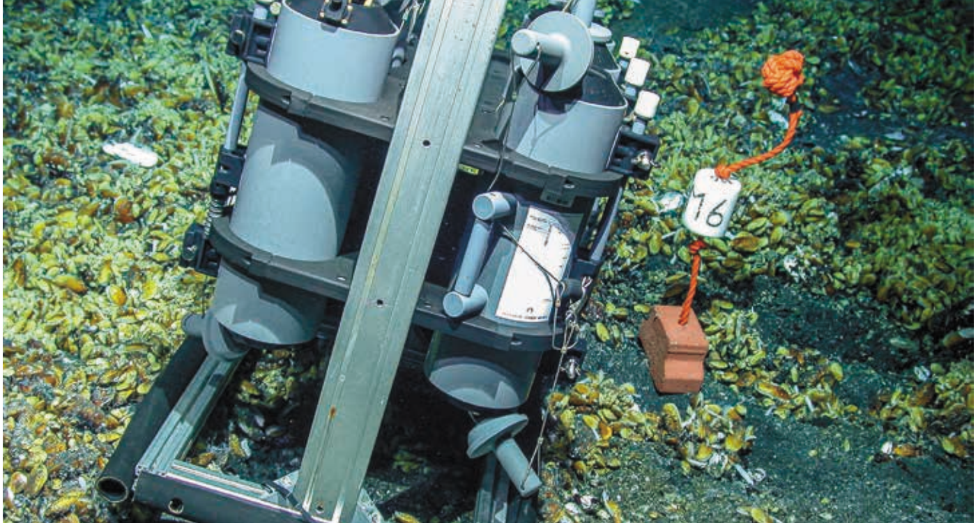
A metal rack housing six open-ended bottles that hold five liters each. LSU oceanographer Jennifer R. Brum uses this equipment to collect virus samples from hydrothermal vents.
