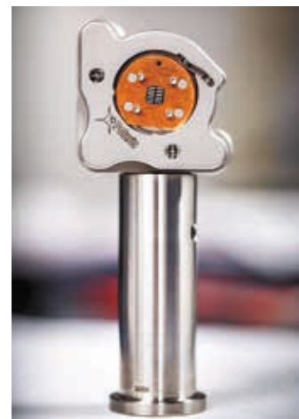
A custom-built device used to measure quantum radiation pressure noise created by LSU physicist Thomas Corbitt and Crystalline Mirror Solutions.
